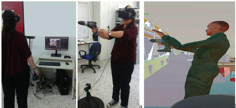
Fig. 5 Riveting in the immersive virtual environment (a) human operator (b) corresponding avatar
