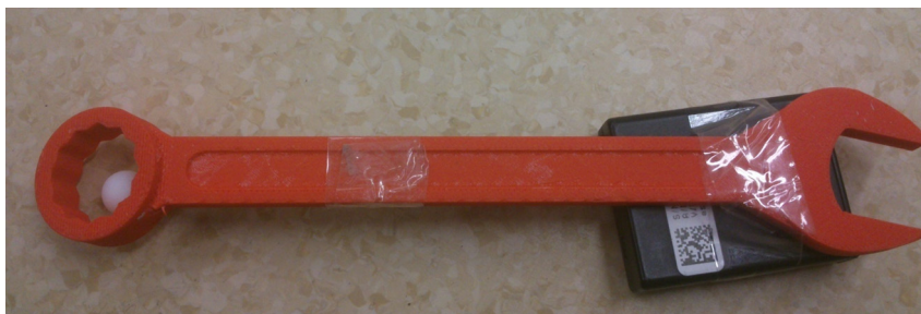
Fig. 11. Physical model of a tool connected with the virtual environment by an optical tracking system marker
