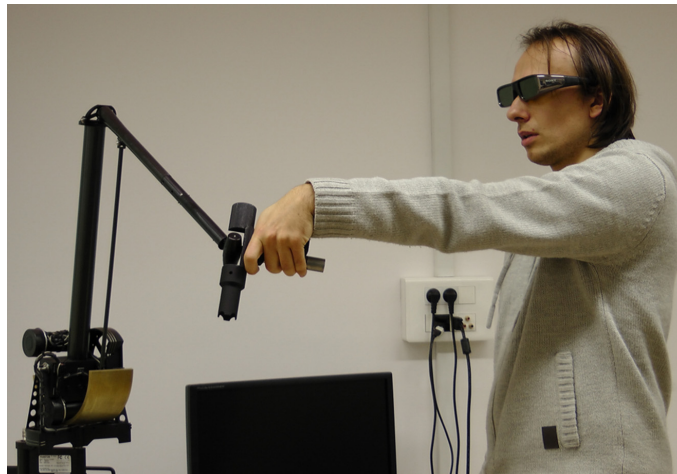
Fig. 9. Manipulation using prototype of the weld gun on a haptic device (visualization realized by stereoscopic large-screen projection system, not included in the photograph)
